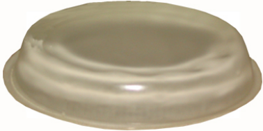
Figure 2 Phase Change Cooling Military Helmet Insert
